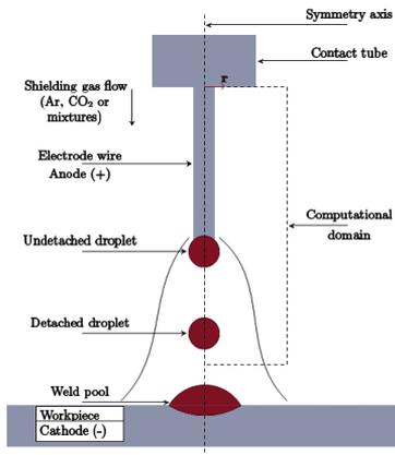
**Figure 1.** Schematic description of gas metal arc welding (GMAW).
